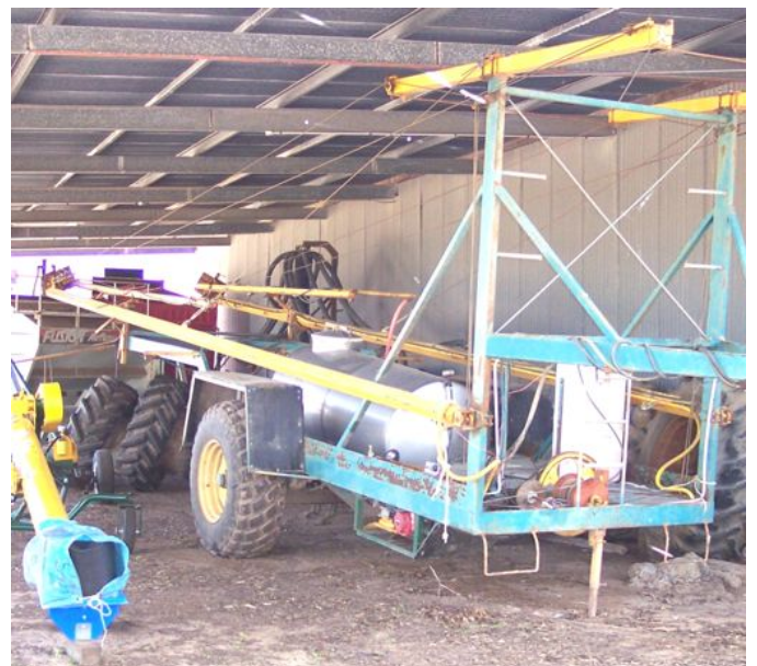
500 spray rig – 37 metre coverage, 120 acres per hour
